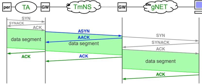
Figure 3: Near-reliable transfer mode
