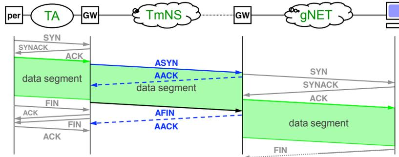
Figure 1: AeroTP connection setup
