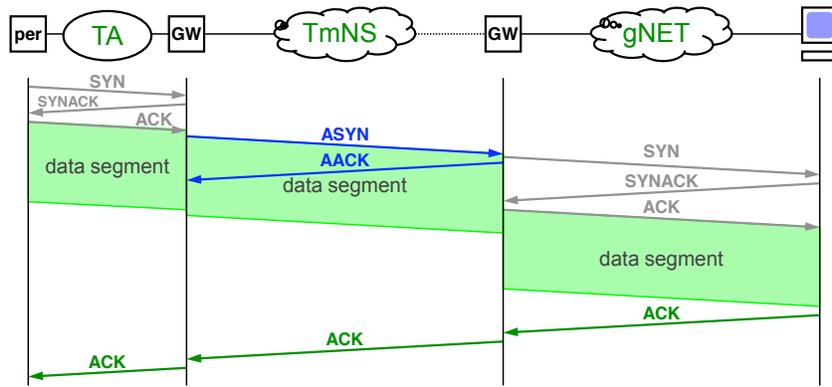
Figure 2: Reliable connection transfer mode
