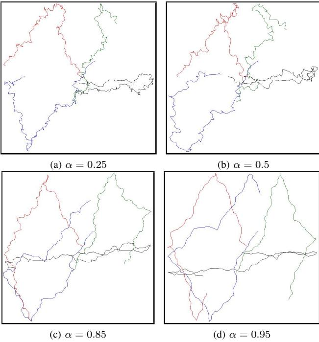
Fig. 3: Gauss-Markov model traces with varying  $\alpha$
