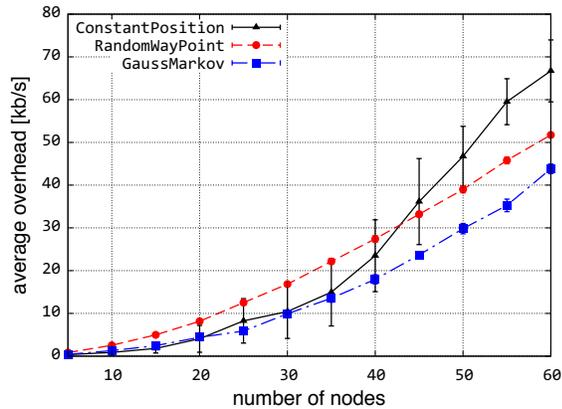
Fig. 7: Effect of node density on protocol overhead
