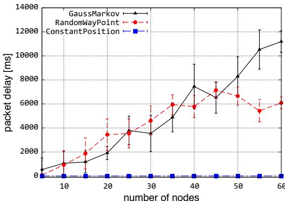
Fig. 8: Effect of node density on packet delay
