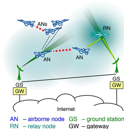
Figure 1. Dynamic airborne telemetry environment
