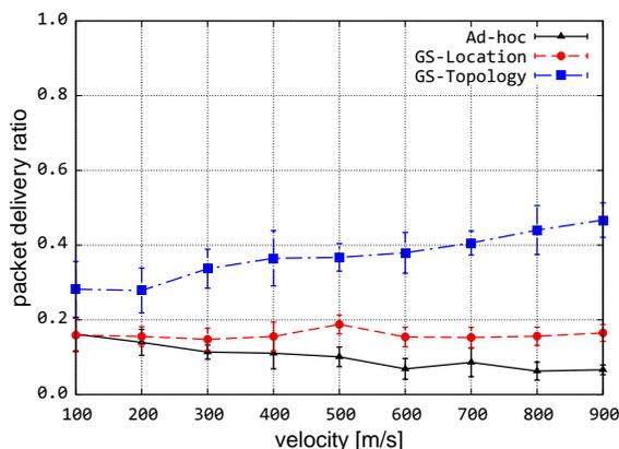
Figure 13. Effect of node velocity on PDR
