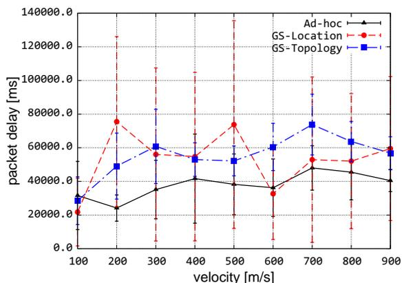
Figure 14. Effect of node velocity on end-to-end delay
