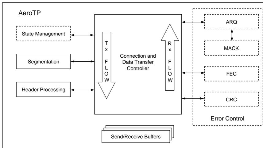
Figure 4. AeroTP implementation architecture
