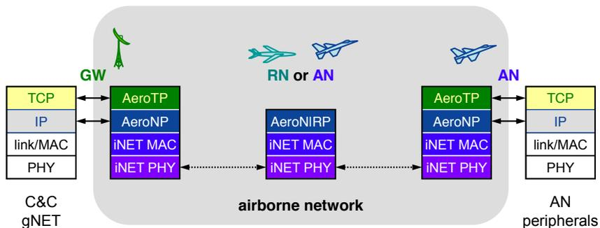
Figure 2. Airborne network protocol architecture
