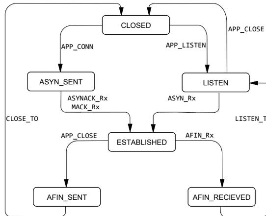
Figure 8. AeroTP state machine
