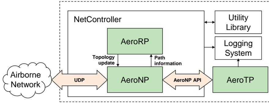
Figure 3. System Architecture
