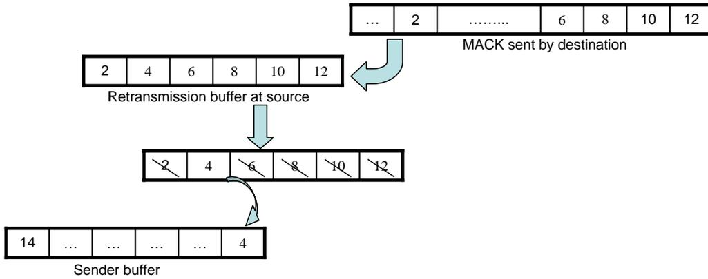
Figure 7. AeroTP ARQ retransmission mechanism
